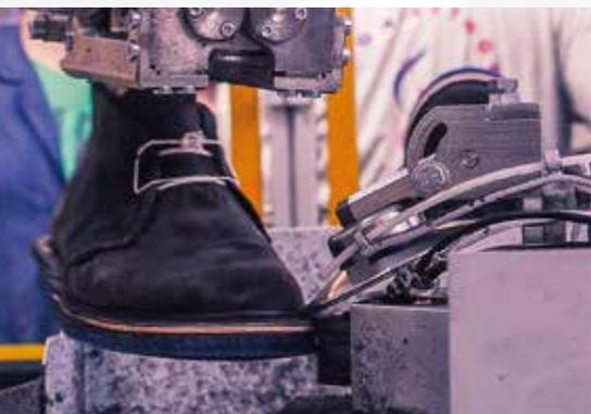
**Robotized workstation for roughing, cementing and milling**
